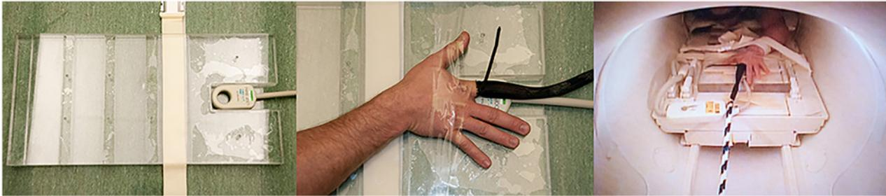
**Fig 1. The radiofrequency coil inside the clear housing (left).** The metacarpophalangeal (MCP) joint of interest centred over the bore of the radiofrequency coil (middle). The participant's hand within the imaging magnet (right).
